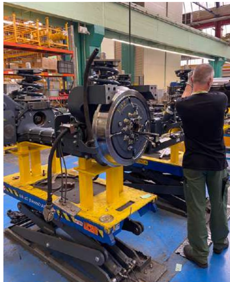
Tramway of Angers - Bogie repair and full servicing within our facilities in Paris
