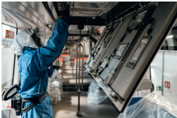
🔗 Maintenance work on a refrigerated ventilation system – metro line 14 train.
