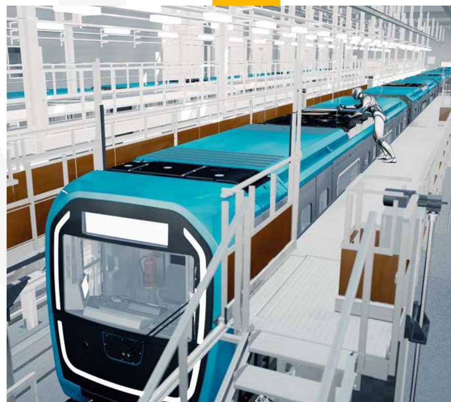
Digital representation of a maintenance centre, simulating a maintenance operation on the upper section of the train.
