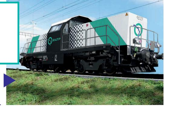
To improve the internal air quality in transport infrastructures, RATP group decided a purchase of 100% electric maintenance shunter for RER works. The shunters are the locomotives used to tow the work trains for the maintenance of the tracks and tunnels.
